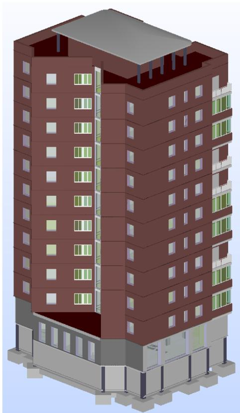
Figure 10: 3D representation of the IFC model of Torre Turina building in Solibri
